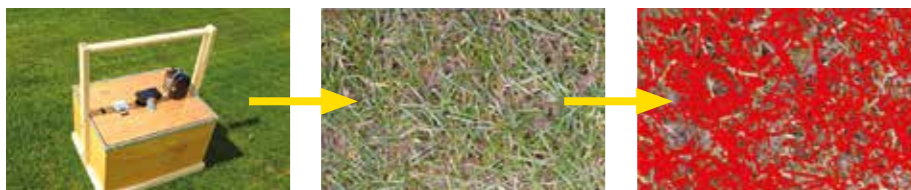
Figure 1 DIA "Digital Image Analysis" process. A digital image is scanned using software to determine "% live ground cover".
